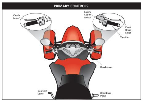
**Handlebars**: Used to control direction of the motorcycle. There is a handgrip on each end.
